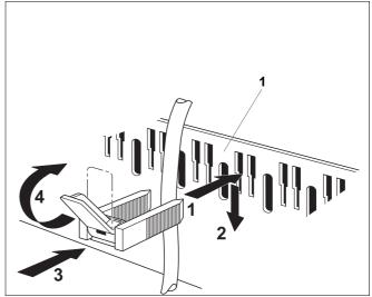
Fig. 16 Secure the cable with a cable clips
