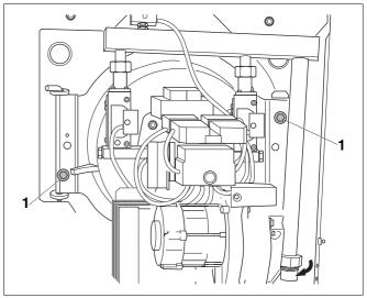
Fig. 23 Burner door SB315 VM with installed pre-mix burner
