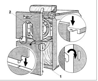
Fig. 25 Install the front panel SB315
