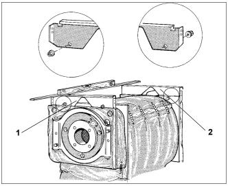
Fig. 7 Install the front and rear support brackets
