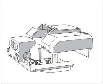
Fig. 20 Install the 2000 control unit
