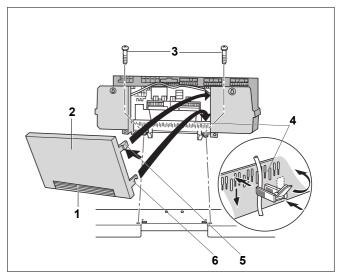
Fig. 15 Remove the rear panel
