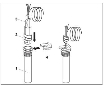
Fig. 18 Sensor well and temperature sensor
