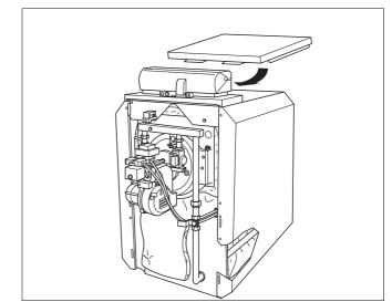
Fig. 24 Install the boiler casing
