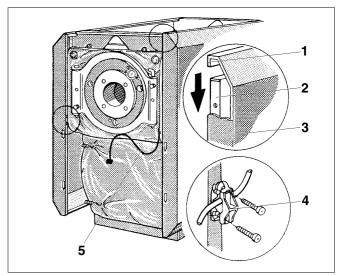
Fig. 10 Fit the strain relief
