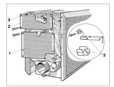
Fig. 11Install the rear wallsItem 1:Lower rear wall sectionItem 2:Upper rear wall section
