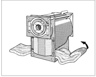
Fig. 4 Installing the thermal insulation
