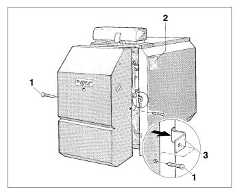
Fig. 26 Install the burner hood SB315 VM
