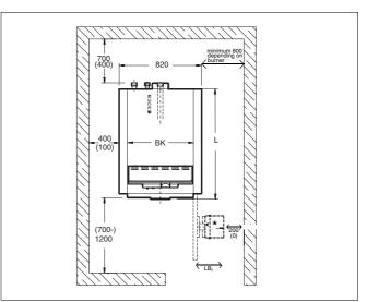
Fig. 3 Location (dimensions in mm, values in brackets () are minimum clearances)
