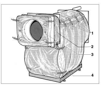
Fig. 5 Fit the thermal insulation
