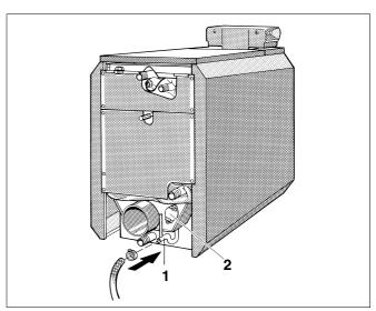
Fig. 27 Fit the drain hose
