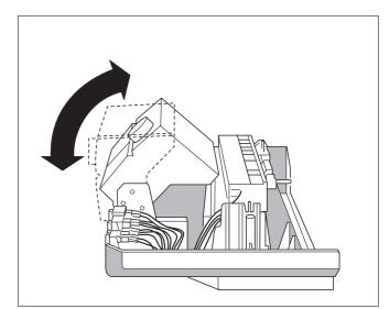
Fig. 19 Pivot the display unit into place
