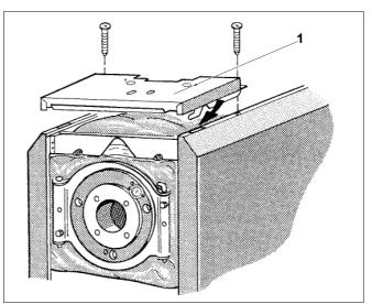
Fig. 12 Install the boiler front cover
