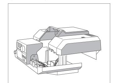
Fig. 14 Install the Logamatic 2000 control unit
