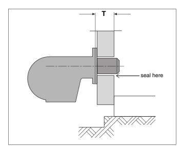
Fig. 22 Schematic diagram of the door depth T
